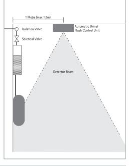
The correct positioning of the PIR sensors depends on assessing the main direction of movement of people under the sensor. These sketches illustrate the principal that the traffic flow should pass through the sensor detection beam.
