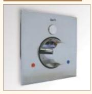
This unique wall mounted bathfiller has an anti-ligature easy-grip temperature control knob, linked directly to a recessed Thermostatic Mixer Valve (Type 3 DO8 NHS Approved). Bathfill is started by a Touch Sensor and stops automatically at the pre-selected level (a tamperproof 'refill delay' setting is optional). Other features can include a divert to shower, and a 1/2 and full fill sensor option – all thermostatically controlled.
